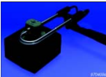
Fig. 6 Pressure calibration made with sound level meter calibrator
